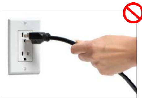
Fig.1- Prohibited to pull the cable
